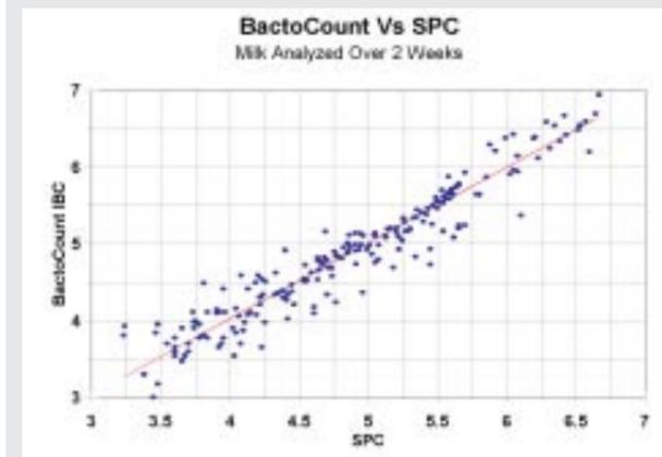
Comparison of the BactoCount IBC and the Standard Plate Count methods for the enumeration of bacteria in raw milk. 209 cold milk samples were simultaneously analyzed over 2 weeks on the BactoCount IBC and by the reference method. The results are expressed in log unit.
