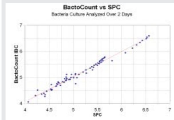
Comparison of the BactoCount IBC and the Standard Plate Count methods for the enumeration of bacteria in raw milk. 69 cold milk samples were spiked with a single culture of bacteria and simultaneously analyzed on the BactoCount IBC and by the reference method. The results are expressed in log unit.
