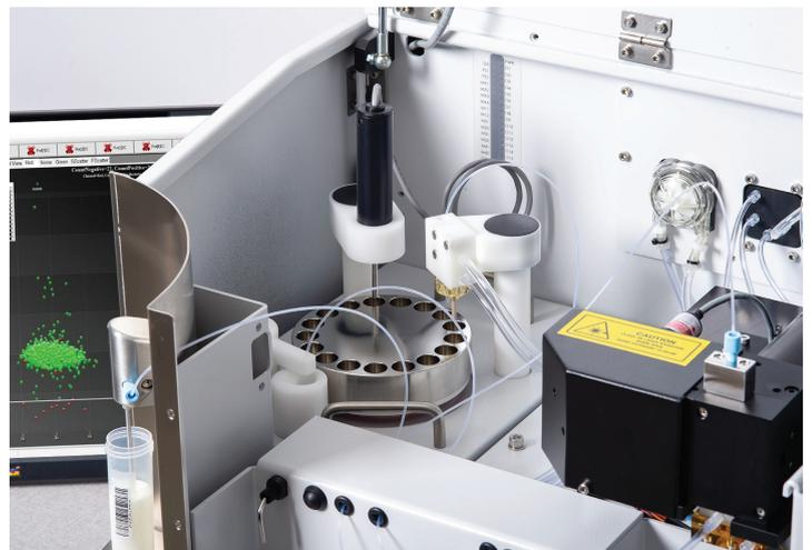
The use of an ultrasonic probe is an important feature for bacteria counting applications. The cavitation effect removes potential interfering components such as somatic cells and gives the method its high sensitivity and Signal-to-Noise ratio. The carousel is automatically cleaned before and after each analysis to eliminate carry-over. The carousel can also be easily removed from the instrument for a more thorough cleaning if necessary.
