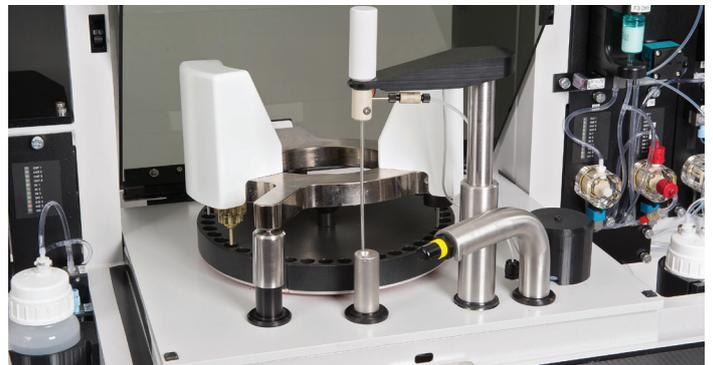
The use of ultrasonic probes is an important option for bacteria counting applications. The cavitation effect removes potential interfering components such as somatic cells and gives the method its high sensitivity and Signal-to-Noise ratio. The carousel is automatically cleaned before and after each analysis to eliminate carry-over. The carousel can also be easily removed from the instrument for a more thorough cleaning if necessary.
