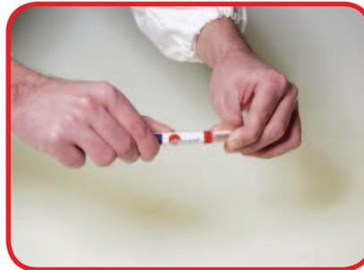
3. break the glass vial contained in the tube by using the clamp cod. 91255
