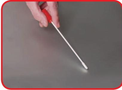
1. take the swab out of the tube and streak on a surface measuring 100 cm<sup>2</sup> (10x10 cm)
