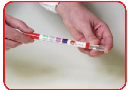
5. evaluate the result after 10 minutes evaluating the result by matching the colour with colorimetric scale
