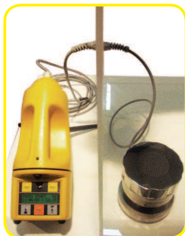
Connection between SAS command unit and aspirating chamber
